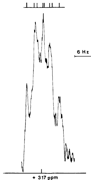
Figure 3. ^{14}N nmr spectrum of I in D_2O at 6.50 MHz with proton stabilization and simultaneous irradiation of the (CH_3)_3N^+ proton signal. The chemical shift is expressed in parts per million (ppm) upfield from the NH_4NO_3 resonance.
